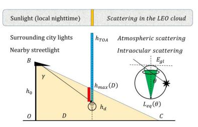
Fig. 1: Sources, media and physical processes involved in the build-up of the artificial sky brightness. Image credit: the Authors.
