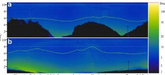
Fig. 1: Stitched high-resolution all-sky images after DiCaLum processing. The luminance heat map shows the panoramic view on a darker woodland field (a) and on a brighter open field (b). The green line indicates the mean vertical sky radiance for green channel radiance (<sub>G</sub>) in the dark sky unit (dsu).
