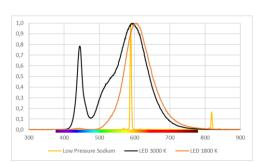
Fig. 1: comparison of the light spectra of three outdoor lighting technologies: 3000K Led (black) / amber 1800K Led (red) / Low Pressure Sodium (orange). @Matthieu Iodice, Cerema
