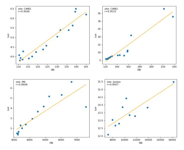
Fig. 2: Correlations between the indoor lux measurements (measured in Lux units) and the outdoor wall brightness extracted from the 360 panoramic images taken on the street level (reported as digital number, DN) taken from various heights from the ground of 4 high-rise buildings in 3 mixed commercial-residential districts in Hong Kong. The DN values were averaged from the RGB channels.
