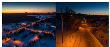
Fig. 1: Fully compliant PC-amber LED streetlights on Mont-Megantic International Dark Sky Reserve municipalities (photo by Guillaume Poulin).
