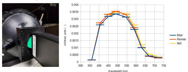
Fig. 1: Left: SQM at the output of the test source.. Right: Spectral responses of the analysed SQMs
