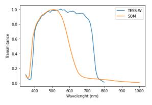
Fig. 1: Spectral response (Transmittance) in function of wavelength of TESS-W and SQM.
