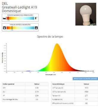
Fig. 1: Screen capture of the data sheet from LSPDD (LED, 1500K).,
