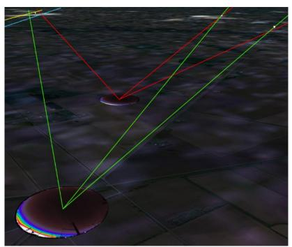
Fig. 1: Test identification of light dome sources via triangulation method. Map Image: Google, Landsat/Copernicus
